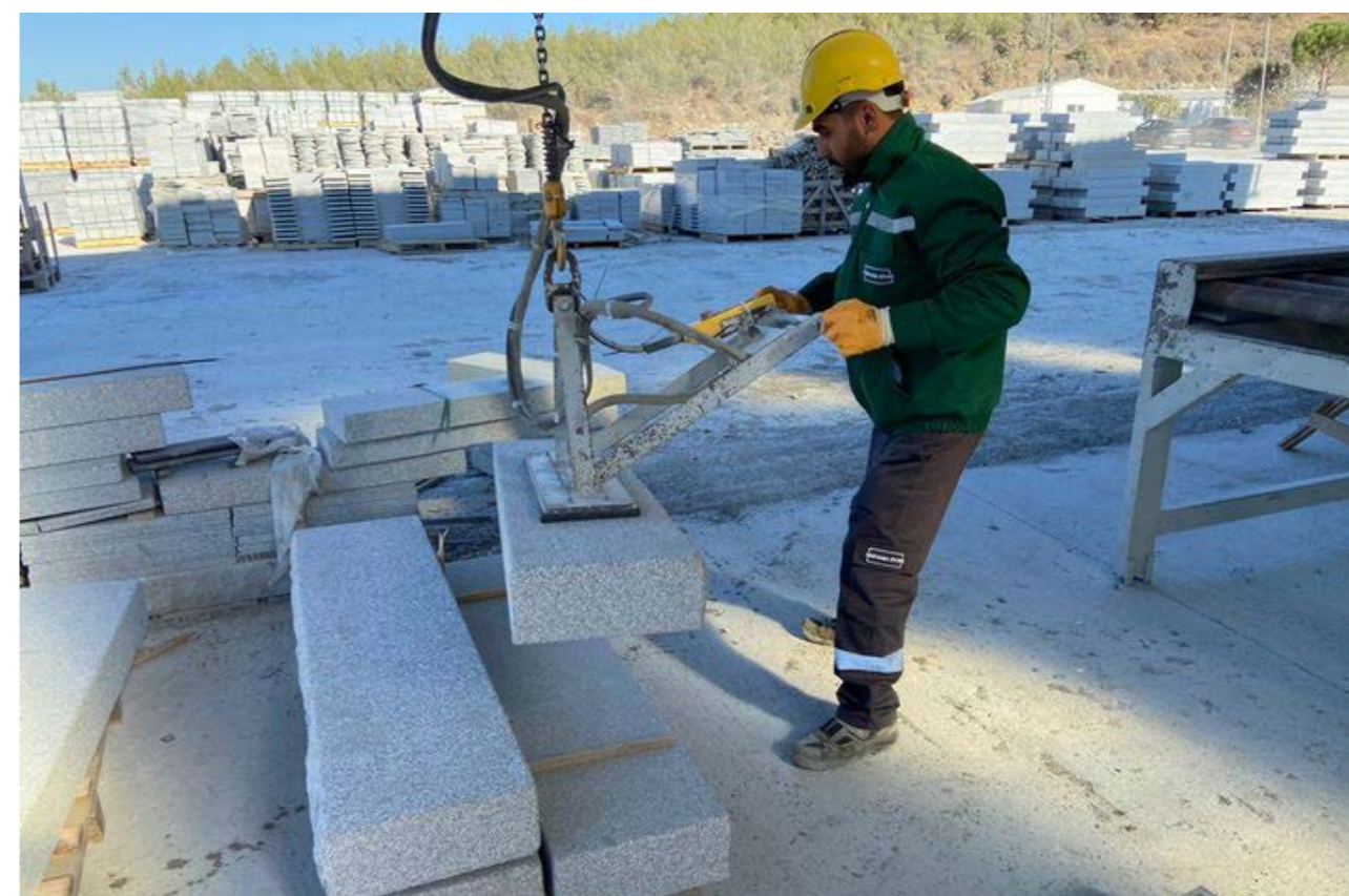
Specialised lifting equipment reduces strain from manual lifting of granite products at Stenbolaget's factory in Bergama, Turkey
